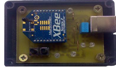
Fig. 5. The designed and implemented coordinator node of the utilized WSN
