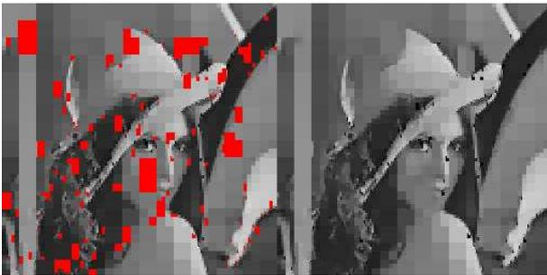
Fig. 8. Applied mask on the lossy image (left side) and results of image inpainting (right side)
