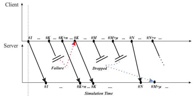
Fig. 2. Phenomena observed during a data packet transmission from Client to Server
