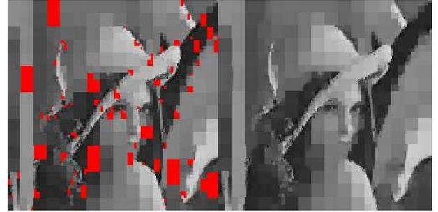
Fig. 10. Applied mask on the lossy image (left side) and results of image inpainting (right side)
