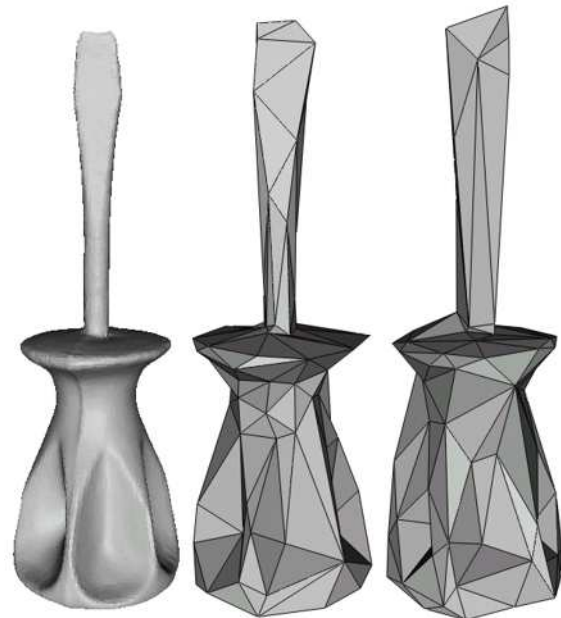
Figure 6: Screwdriver: Initial model (54,300 faces), hulls of 200 faces generated with the 1st and 2nd strategy respectively.
