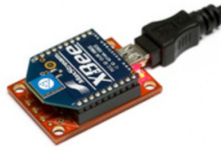
Fig. 4. The designed and implemented coordinator node of the utilized WSN
