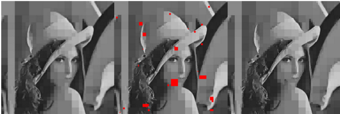
Fig. 8 The L=0.3 QT-decomposed image (left side), the masked received lossy image (middle portion) and the resulting repaired image 4–levels(1.2 sec), N = 12 (right side)
